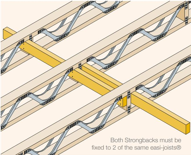
Both Strongbacks must be fixed to 2 of the same easi-joists®
