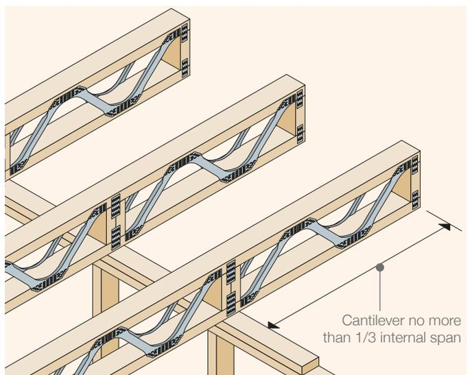
Cantilever no more than 1/3 internal span
