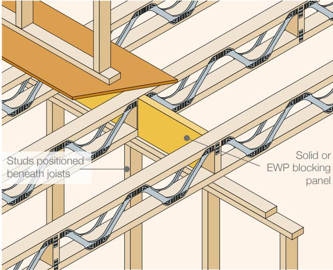
**T4 • Intermediate Support (on to stud wall)**
