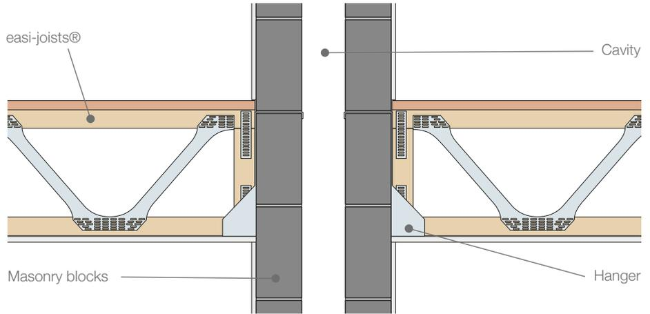
Both the floor decking and plasterboard to the underside of the **easi-joist®** are required to extend to the masonry block.
