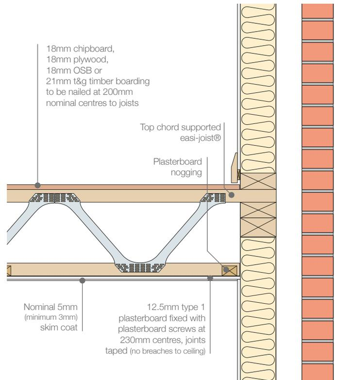
Intermediate Floor Construction: 30 minutes Fire Resistance with **easi-joists®** at 400mm Centres
