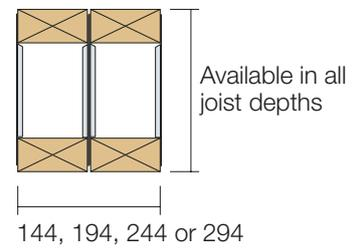
easi-joist® metal web joists are available in 6 different depths utilising 35mm and 47mm top and bottom timber chords.
