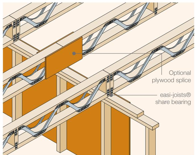
**T3 • Intermediate Support Bearing Over Stud Wall**
