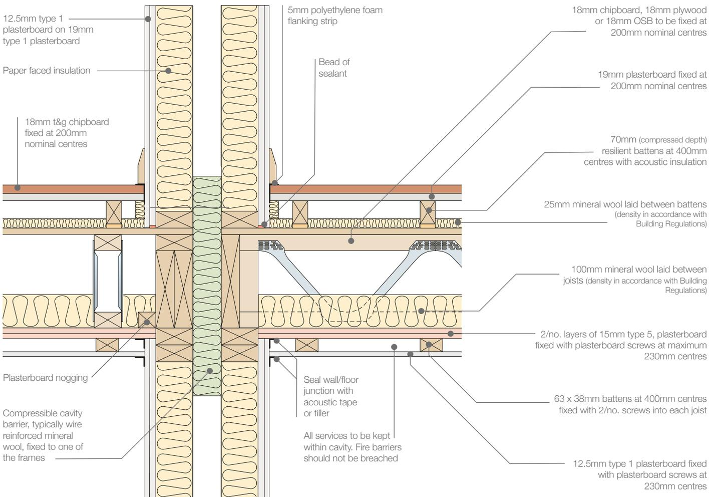
Separating Floor Construction: 60 minutes Fire Resistance
