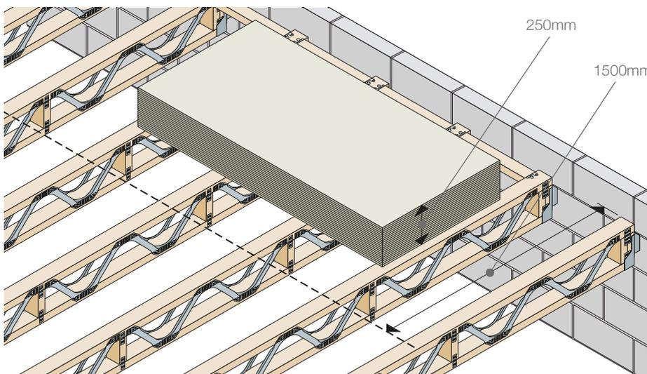
**IMPORTANT:** It is inadvisable to stack building materials on floor joists other than floor decking as described above.
