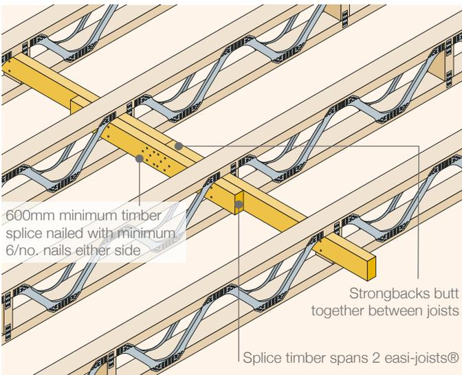
600mm minimum timber splice nailed with minimum 6/no. nails either side
