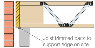
When trimming ensure a minimum of 50mm gap to the end of a metal web or plate
