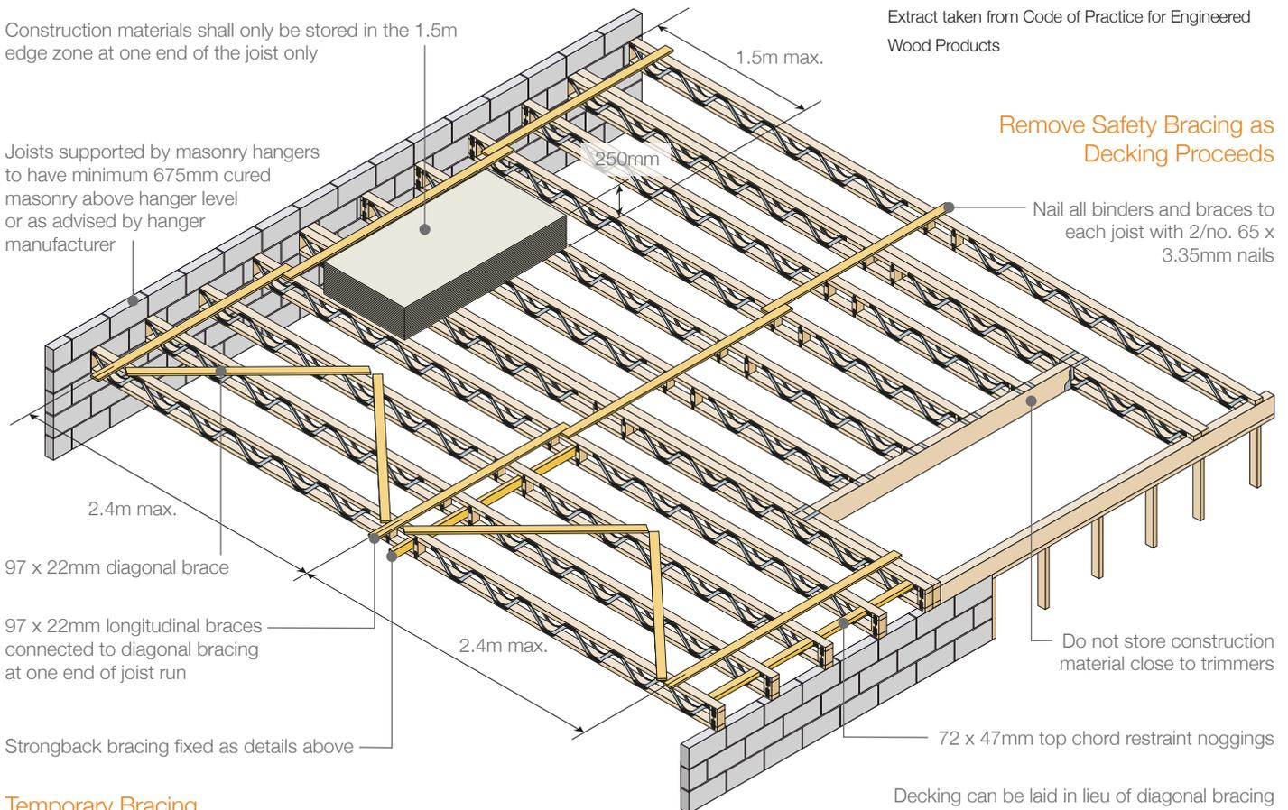
Decking can be laid in lieu of diagonal bracing
