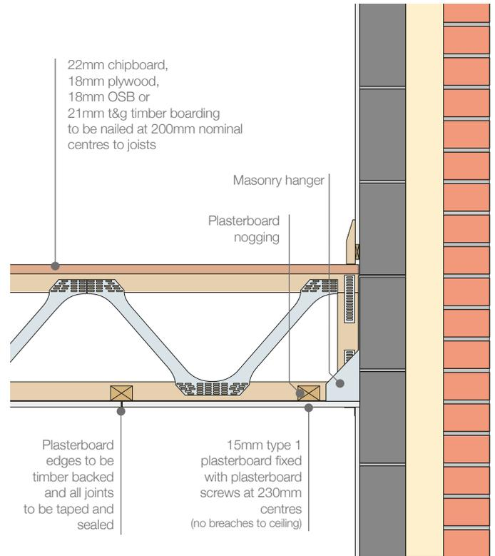
Intermediate Floor Construction: 30 minutes Fire Resistance with **easi-joists®** at more than 400mm Centres
