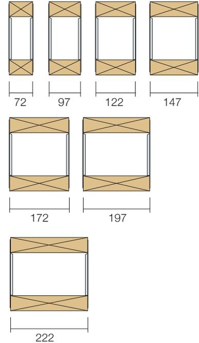
Multi-ply joist widths
