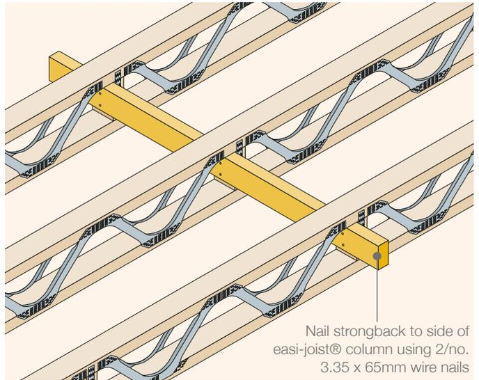
Nail strongback to side of easi-joist® column using 2/no. 3.35 x 65mm wire nails
