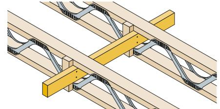
Fix 97 x 35mm (min) strongbacks to joists with 2/no. 65 x 3.35mm wire nails.
