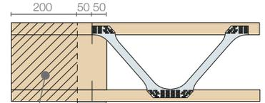
Trimmable section Remaining blocking and easi-joist not to be trimmed
