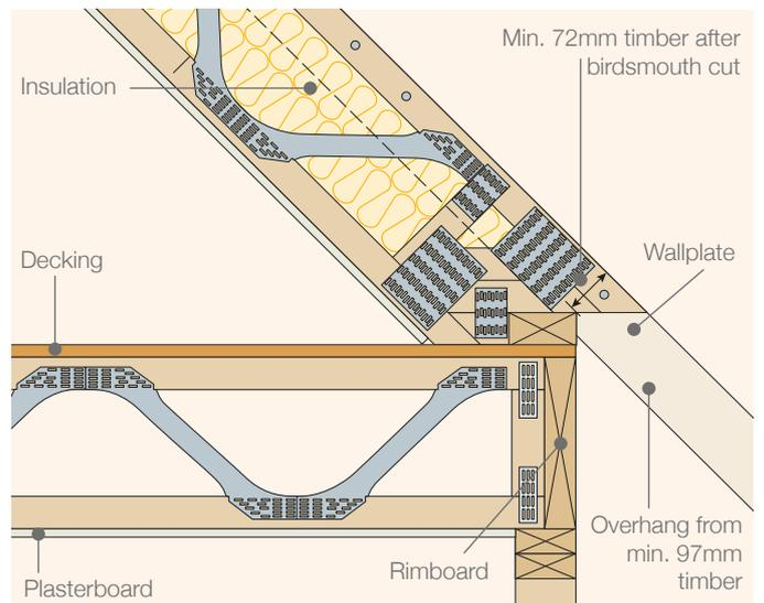
The flexibility of putting **easi-joist®** in a truss goes beyond adding to its strength properties. Insulation thickness has grown and is a potential problem for home owners wishing to use the attic space for storage. Adding **easi-joist®** into the truss overcomes this issue by raising the attic floor level and providing adequate space for the insulation.
