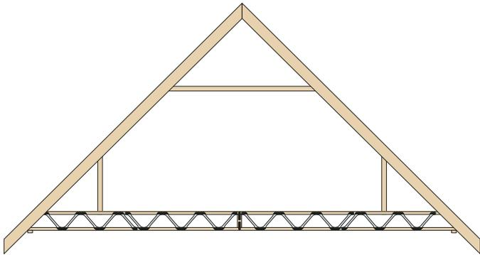
**easi-joist®** can be designed in a truss in a variety of ways. The most common use is within an attic truss forming the bottom chord section. It can also be designed only within the floor zone depending on the requirements.
